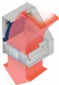
High fan speed, air valve is entirely open to retain the low air velocity.
